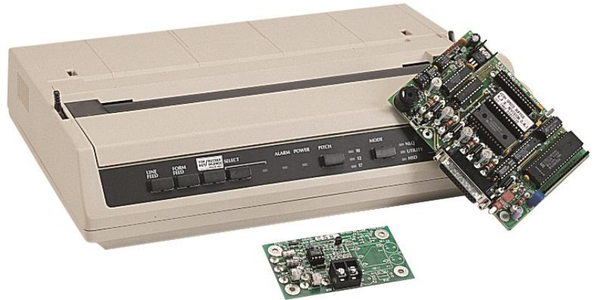
Remote Line Printer with the Internal controller board and System 3505 Prism Lx Interface board.
