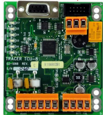
Qnode Controller PCB
